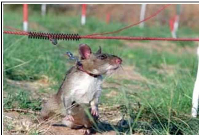
The mine-detection rat is harnessed and linked to the search line. Two leashes are connected to the glider to allow manipulation of the animal's position in the box from the safe lanes.
